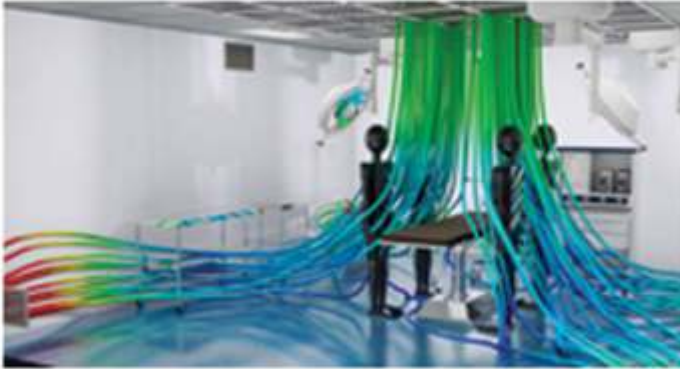
Laminar flow pattern inside an Operating Room
